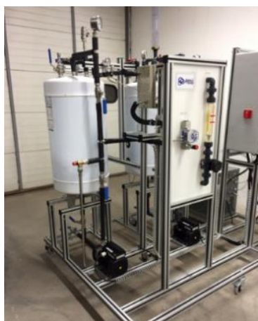
Figure 112. Bench-scale unit for testing membranes on isobaric MD.
