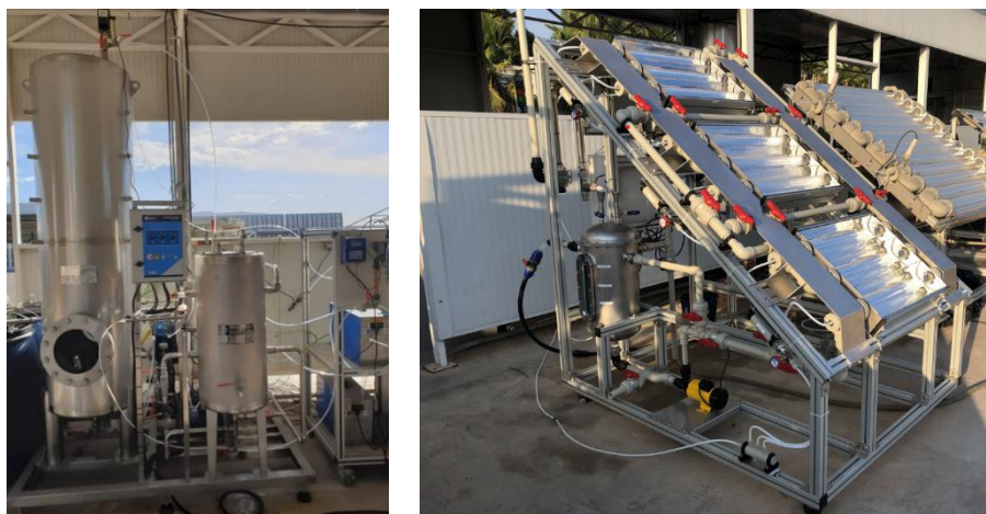
Figure 36. Ozone (left) and solar CPC reactor (right) pilot plants used in Andromeda for assessing novel photocatalytic materials for water purification.
