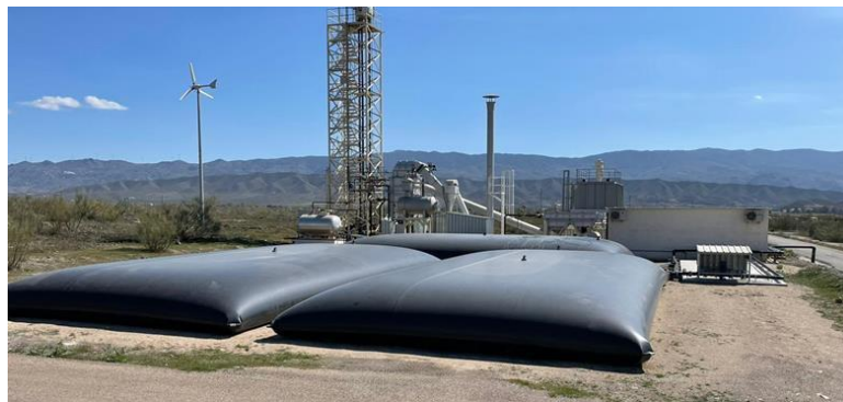
Figure 79. Containers filled with real seawater for desalination tests in closed loop.
