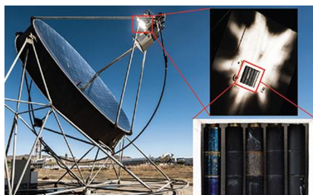
Figure 66. Accelerated aging tests of steel samples at a parabolic-dish DISTAL- II
