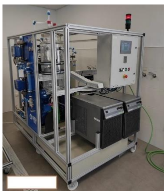
Figure 97. MD + crystallizer pilot plant developed by Apria Systems S.L.
