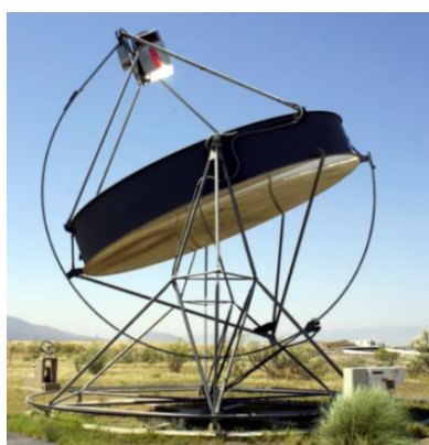
Figure 65. View of a parabolic-dish DISTAL- II with the original Stirling engine.
