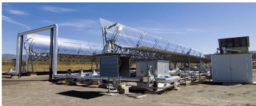
Figure 49. View of the IFL experimental facility (with parabolic troughs) using compressed gas as heat transfer fluid.
