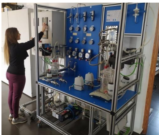
Figure 114. Bench-scale unit for testing FO and PRO.
