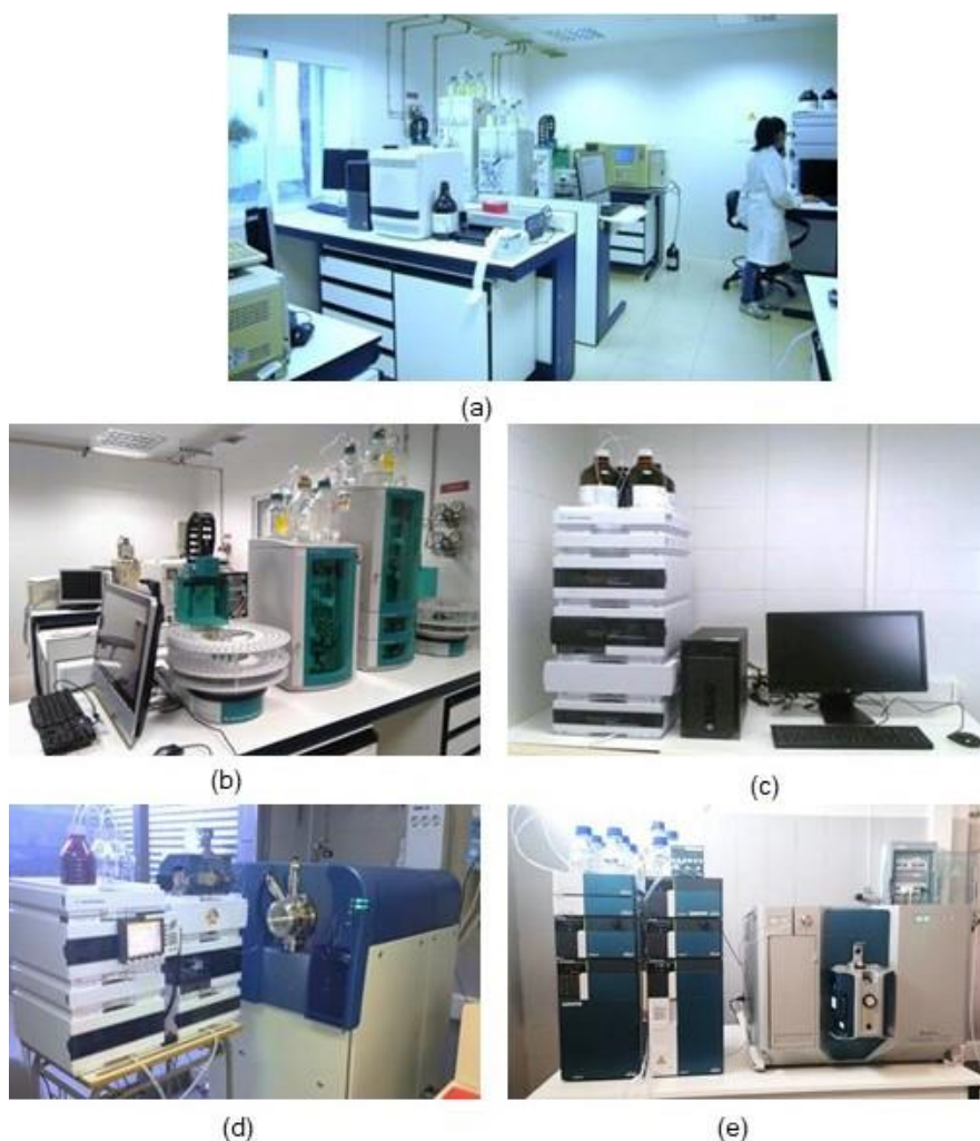
Figure 116. (a) General view of the chromatography lab at PSA facilities. (b) Metrohm Ion Chromatographic System. (c) Agilent Ultra-fast UPLC-DAD analyzer. (d) AB SCIEX TripleTOF 5600+ equipment. (e) AB SCIEX 7500 QTRAP Ready LC/MS.
