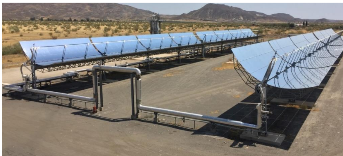
Figure 11. PROMETEO test facility used at PSA for HELISOL®XLP proof of concept.
