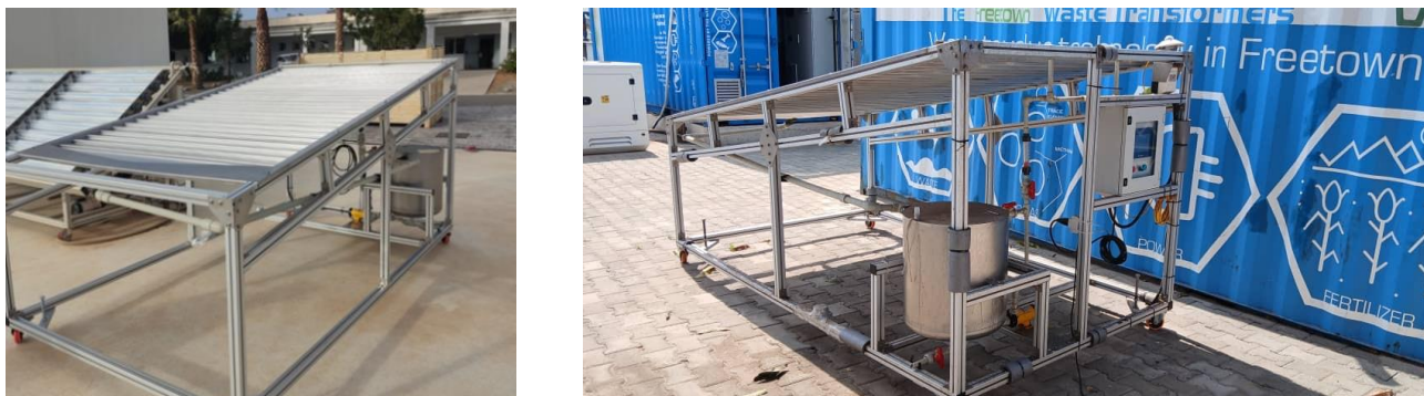
Figure 31. MSCR of ENERGICA for water treatment: (left) pilot plant of 50 L containing \text{TiO}_2 immobilized in stainless steel stairs at CIEMAT facilities and (right) MSCR installed in Sierra Leone.
