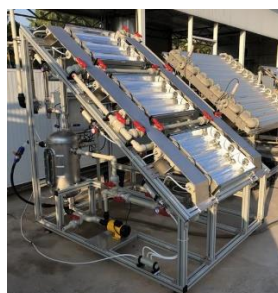
Figure 90. Solar CPC with direct injection of ozone available at PSA facilities
