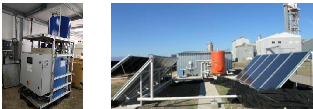
Figure 76. Internal (Left) and external (right) views of the Membrane Distillation experimental test bed within the PSA low-temperature solar thermal desalination facility.
