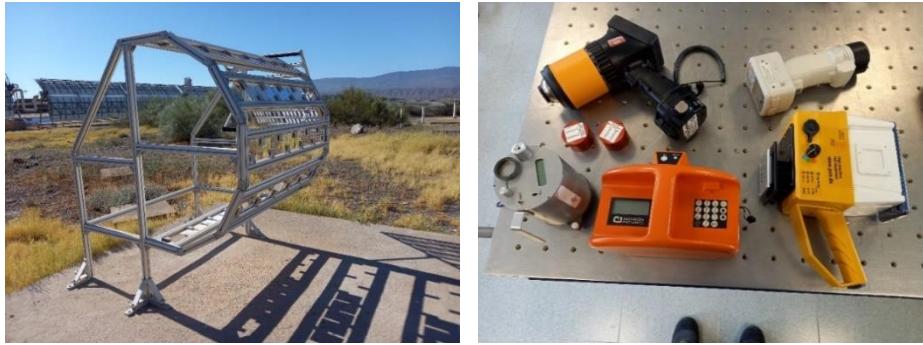
Figure 20. Reflector samples exposed at different inclinations to achieved several soiling levels (Left). Portable reflectometers included in the study of the transfer functions (Right).
