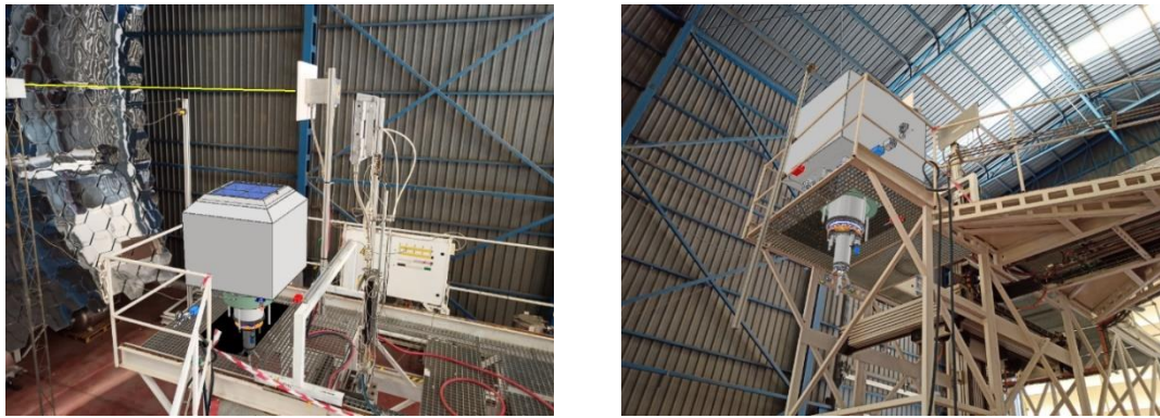
Figure 29. Simulated view of the Sunson-Box on the test platform of PSA's Solar Furnace SF60, seen from above (left) and below (right). Note the opening in the floor needed for the vertical movement mechanism.
