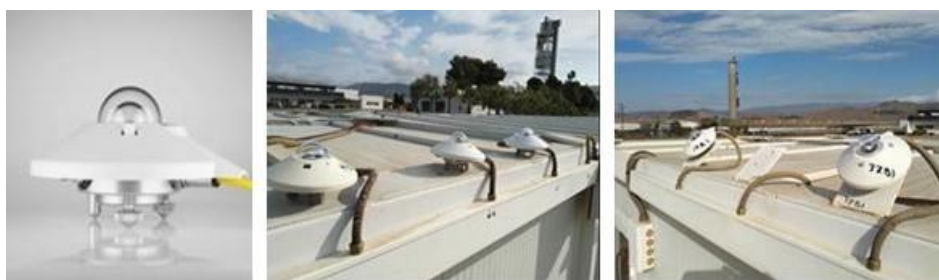
Figure 95. CUV-5 radiometer (left). View of all solar UV radiometers, horizontal (centre) and inclined (right) setup used in the Solar Treatment of Water Unit.
