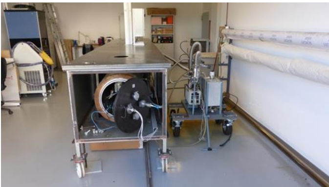
Figure 101. View of the HEATREC test chamber to measure heat losses in solar receiver tubes (left) and RESOL test bench to measure the receiver's optical efficiency (right).
