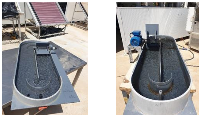
Figure 84. Raceway Pond Reactor with capacities of: (left) 15 L and 5 cm of liquid depth and (right) 90 L and 15 cm of liquid depth.
