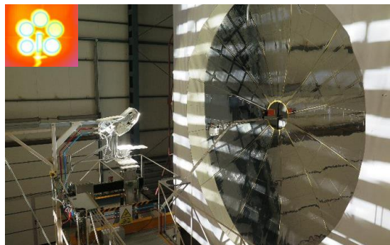
Figure 22. Ageing testing of silicon carbide (SiC) samples SiC) under high concentrated solar fluxes at CIEMAT-PSA's SF40 Solar Furnace. (Left-up) Infrared image of SiC samples at 1,200 °C
