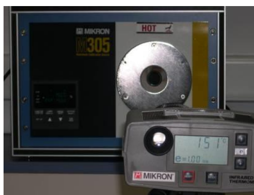
Figure 104. IR sensor calibration using a black body.
