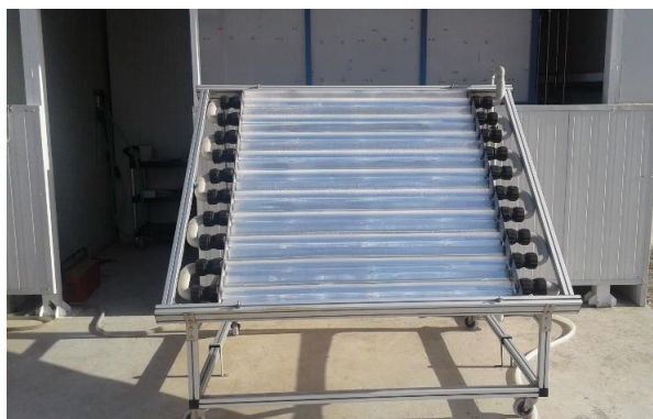
Figure 82. View of 2 m 2 -CPC coupled to Electro-Fenton pilot plant (ELECTROX).
