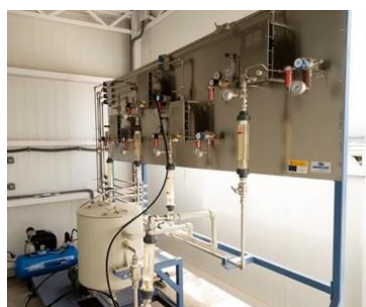
Figure 94. Electro-oxidation pilot plant (left); Electrochemical cell of the solar-assisted electrooxidation pilot plant (centre) and schematic diagram of the solar-assisted electrooxidation pilot plant (right).
