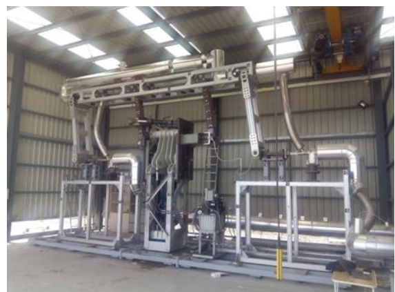
Figure 53. Schematic diagram of the REPA test loop at PSA (left) and north view of the test facility with two flex-hoses mounted for testing (right).
