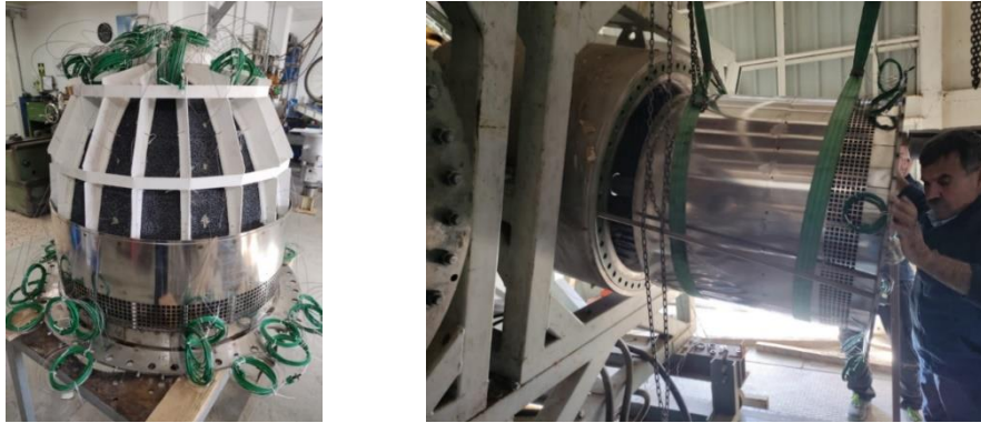
Figure 24. Left. New nickel ferrite absorber. Right: Installation of the absorber within the reactor.
