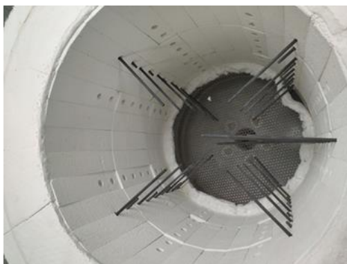
Figure 63. Picture taken from the top of the tank, showing its internal room and thermocouples at different lengths and radial positions.
