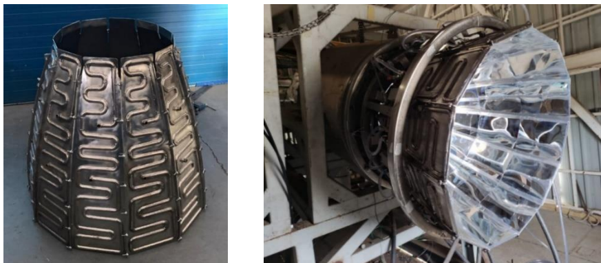
Figure 25. New secondary steel concentrator with an improved cooling system.
