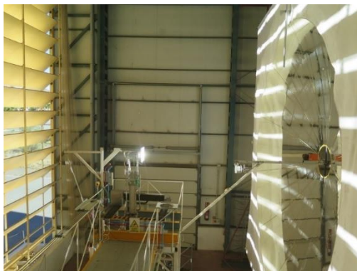
Figure 27. Thermal cycling of samples at the focal zone of the SF-40 at PSA
