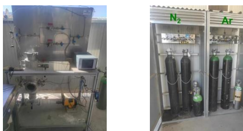
Figure 92. Solar pilot plant for photocatalytic generation of hydrogen (left) and gas (N 2 and Ar) conduction systems (right).
